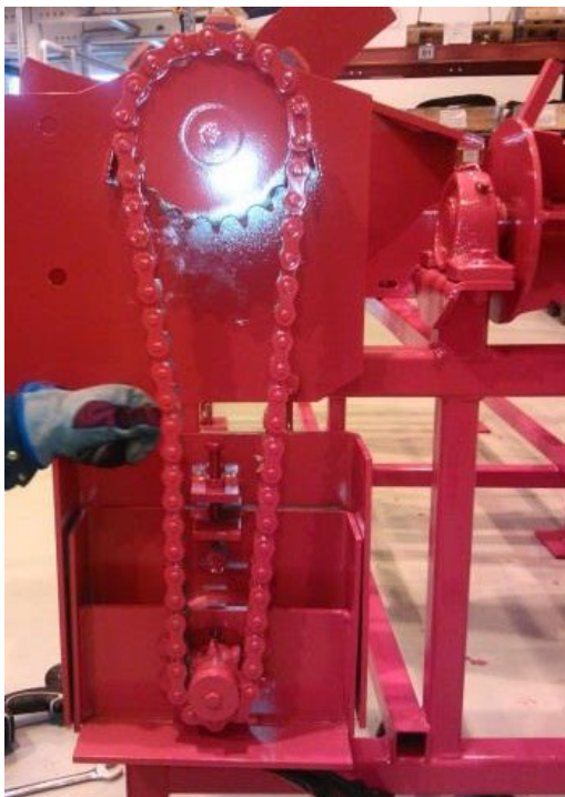
Figure 8. Motor chain lubrication
