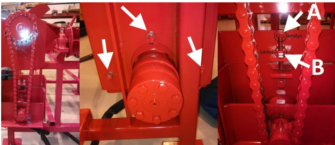
Figure 6. Tightening the motor chain
