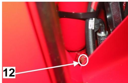
13. Upper nipple for the cutting flange cylinder (only in the Easy model)
