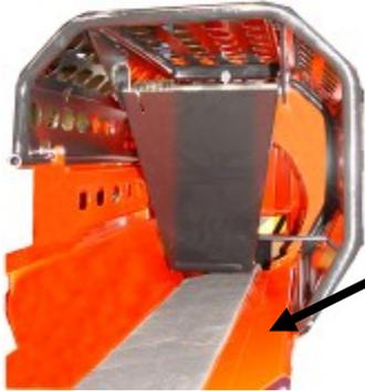
The wood press keeps the logs in place when they are being sawed. Do not put your hand between the wood press roller and the input conveyor belt!
