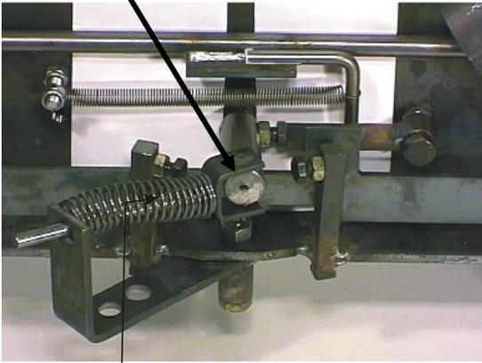
2. The spring presses the jointed lever to the right.
