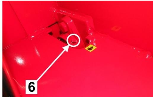
7. Grease nipple for the main shaft bearing (saw side)
