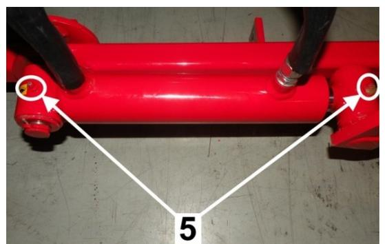
6. Grease nipple for the input conveyor's drive roller
