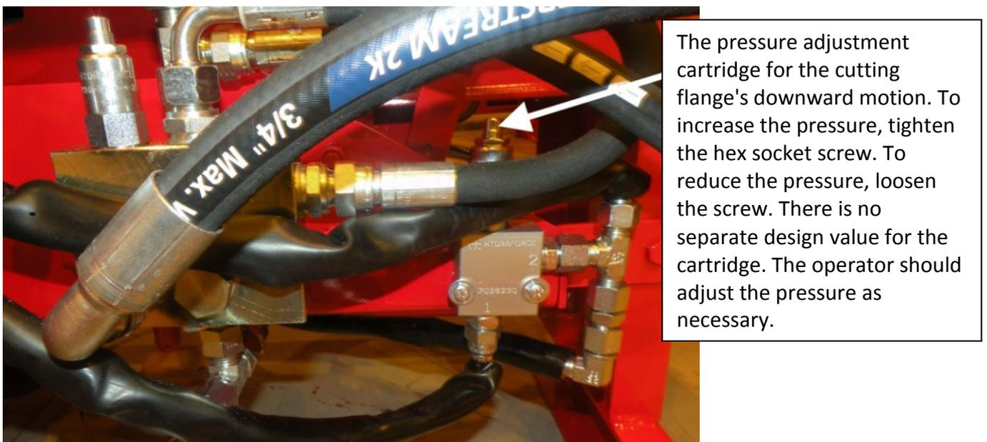
The pressure adjustment cartridge for the cutting flange's downward motion. To increase the pressure, tighten the hex socket screw. To reduce the pressure, loosen the screw. There is no separate design value for the cartridge. The operator should adjust the pressure as necessary.
