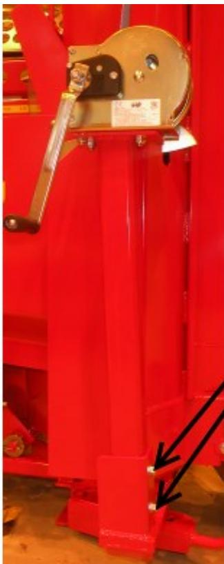
Install the winch support, place the winch (no. 11 in Figure 2) in its slot and tighten the bolts (2 pcs).
