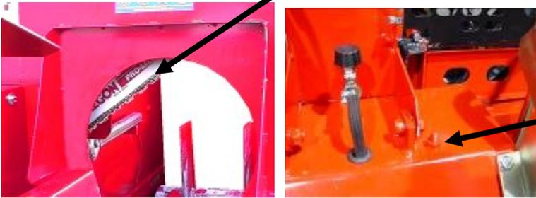
If the blade is not completely raised, tighten the spring pulling the blade by turning its adjustment nut. If the adjustment is not enough, replace the spring.
