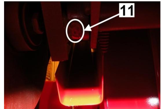
11. Inner nipple for the drive end shaft
