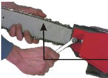
3. Lift the flange and tighten the fastening bolts. Then, lower the guards and lock them in place.
