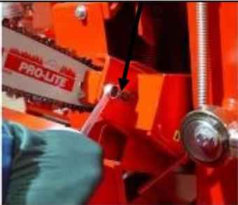
2. Use the adjustment screw to adjust the blade chain. The chain is at the correct tension when pulling the chain fully displays one of the lower teeth.
