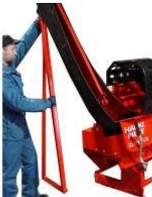
3. Lower the conveyor to a horizontal position, and insert the conveyor support in the slots in the lower section of the machine's frame.
