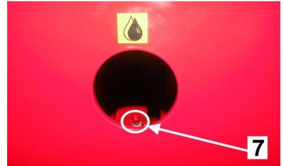
8. Upper nipple for the cutting lever's adjustment rod
