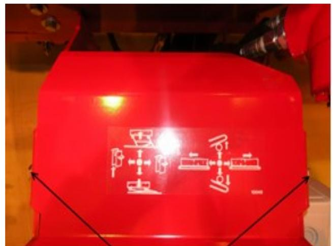
Attach the valve guard to the control panel with two bolts as shown in the figure.
