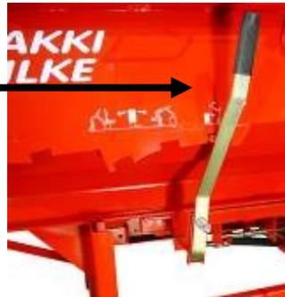
**IMPORTANT!** Using the machine is strictly prohibited if the splitter's operating lever is in the RUN position and the guard of the splitting section can be opened! The faulty locking mechanism must be repaired immediately. It should only be possible to open the guard of the splitting section
