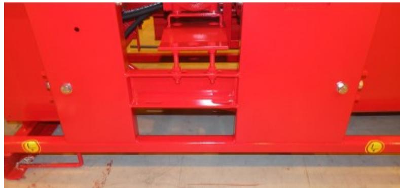
Figure 3. Lifting points for a forklift.
