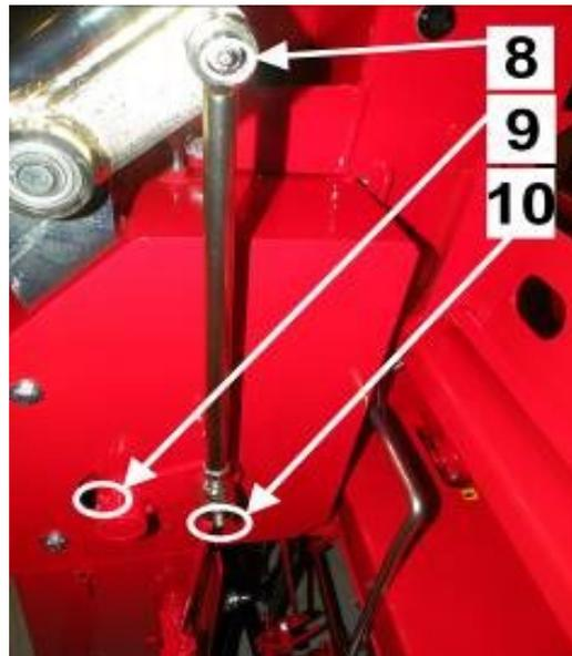
9. Outer nipple for the drive end shaft
