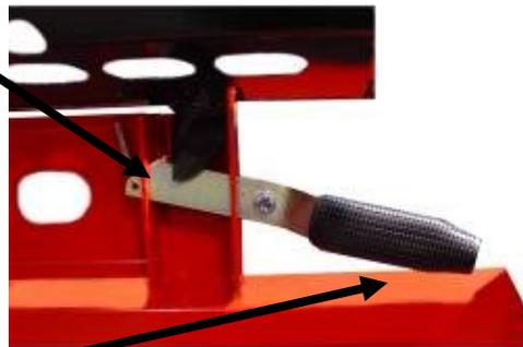
To close the input conveyor guard, push the guard backwards and release the lock. Lower the guard.
