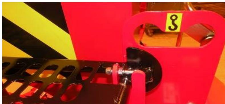
Figure 4. Lifting points for a chain or strap.
