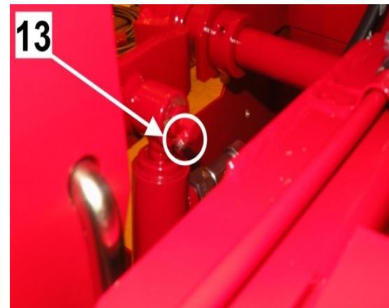
In other words, there is a maximum of 14 lubrication points (Easy model with a pivoting output conveyor). All of the points must be lubricated with vaseline roughly every 10 hours.
