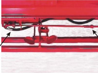
Moving the right-hand stopper adjusts the return motion of the splitting beam, i.e. how close to the splitting blade the splitting beam is brought.
