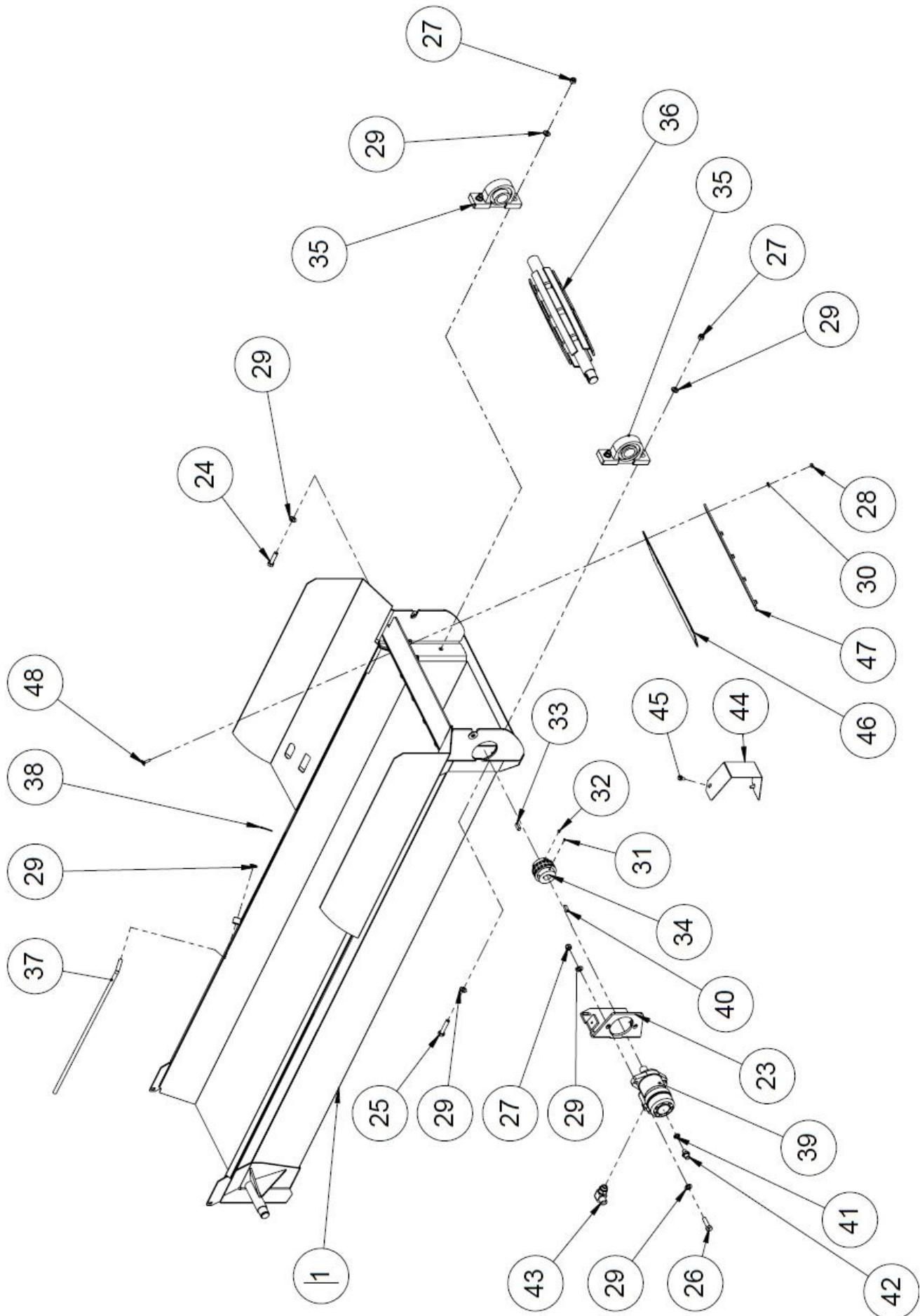
7 Parts list of the lower section of the out-feed conveyor (larger conveyor, 50030190)
