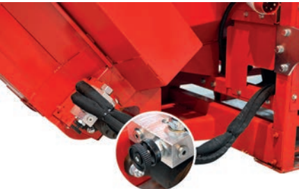
Outfeed conveyor speed control valve as easy-to-install accessory comes as standard equipment.
