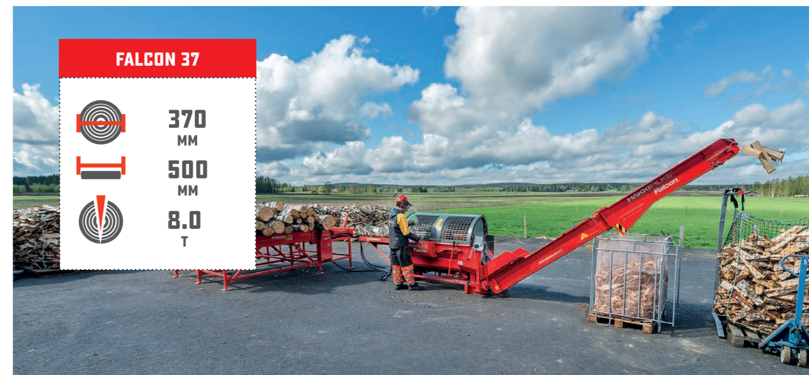
Effective hydraulic saw with automatically optimised saw lowering speed.
