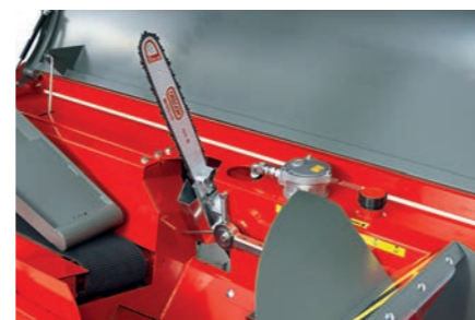
Effective hydraulic saw with automatically optimised saw lowering speed.
