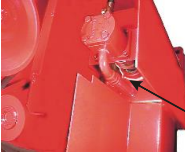
The bearings of the hydraulic pump drive shaft.
