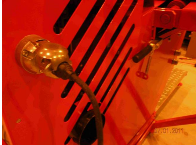
Figure 13. Connector of the optical measuring device
