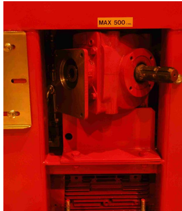
Figure 23. Replacing the angle transmission
