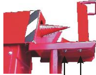
The distance of the rack from the cone can be adjusted with the nuts below the rack
