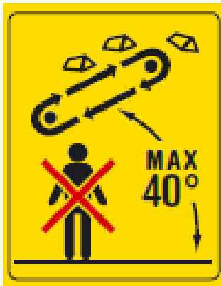
The maximum permitted angle of the conveyor is 40°. Do not walk under the conveyor.
