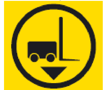
Lifting point for a forklift.
