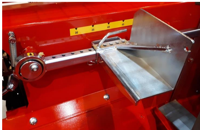
Figure 15: Measuring device position for large logs of more than 25 cm in diameter
