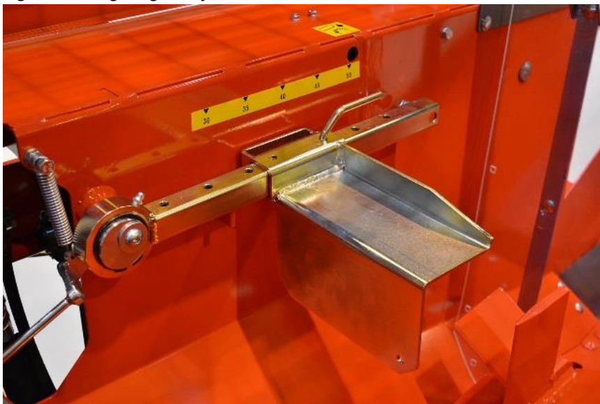
Figure 19. Limiter plate position for smaller logs
