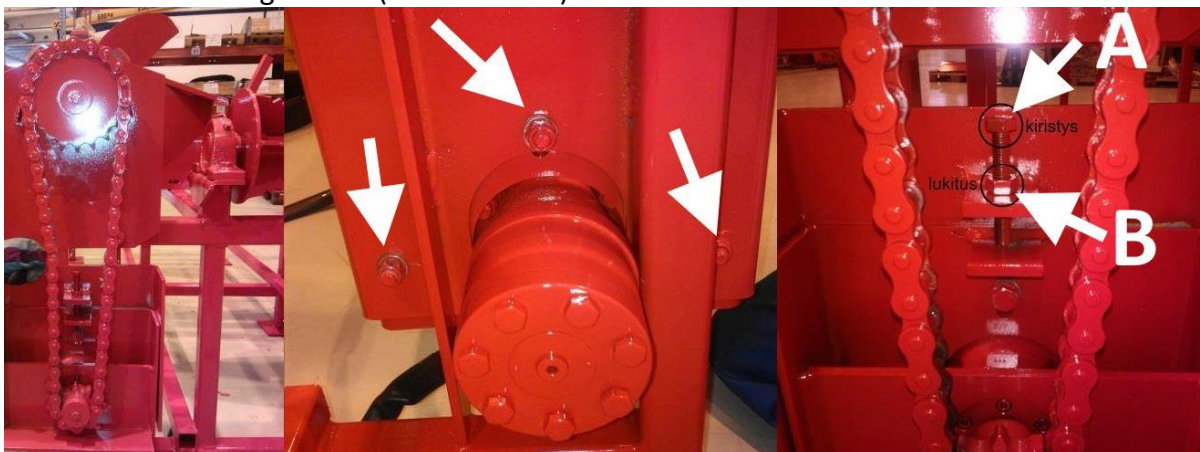
Figure 5 (tightening the motor chain)
