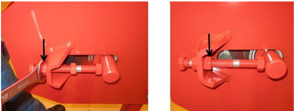
Figure 4 (Arrow left: tension, Arrow right: lock nut)
