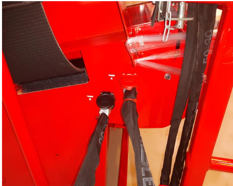
Figure 3. Connecting the hydraulic hose to the machine.
